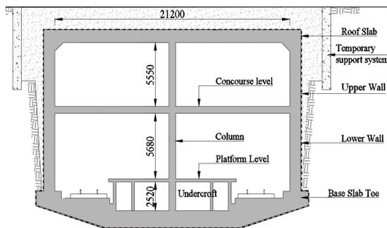
**Fig. 1. Underground Station– typical Elevation.**
